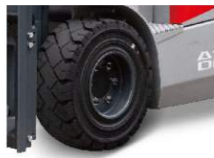
Low rolling resistance electric truck special solid tire reduces driving resistance consumption.
