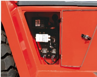
Independent integrated electric cabinet
