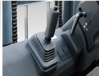
Ratchet type parking brake
