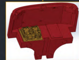
The electric control is placed on the counterweight
